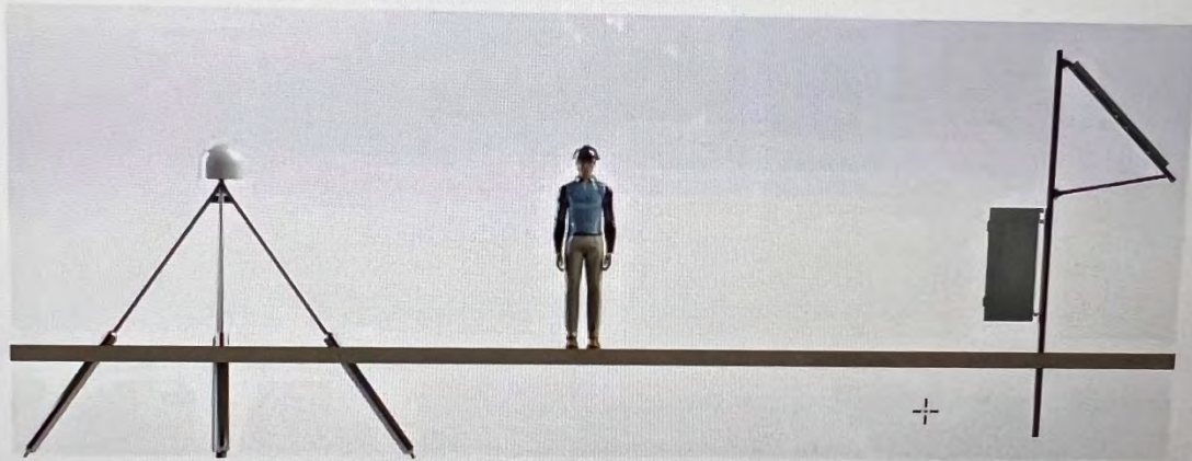
Figure 2. The quincunx deep-drilled braced monument with associated power system. Components are included in the DDBM Station Components line item in the budget (Appendix 1): stainless steel pipe for the monument, radome and antenna mount assembly, liquidtite, cabling, fittings, enclosure with 4x 12 volt 100 amp/hr batteries, standard backpanel, 180-220 watt solar array, cellular telemetry kit, upgraded grounding and surge suppression compared to PBO-spec.
