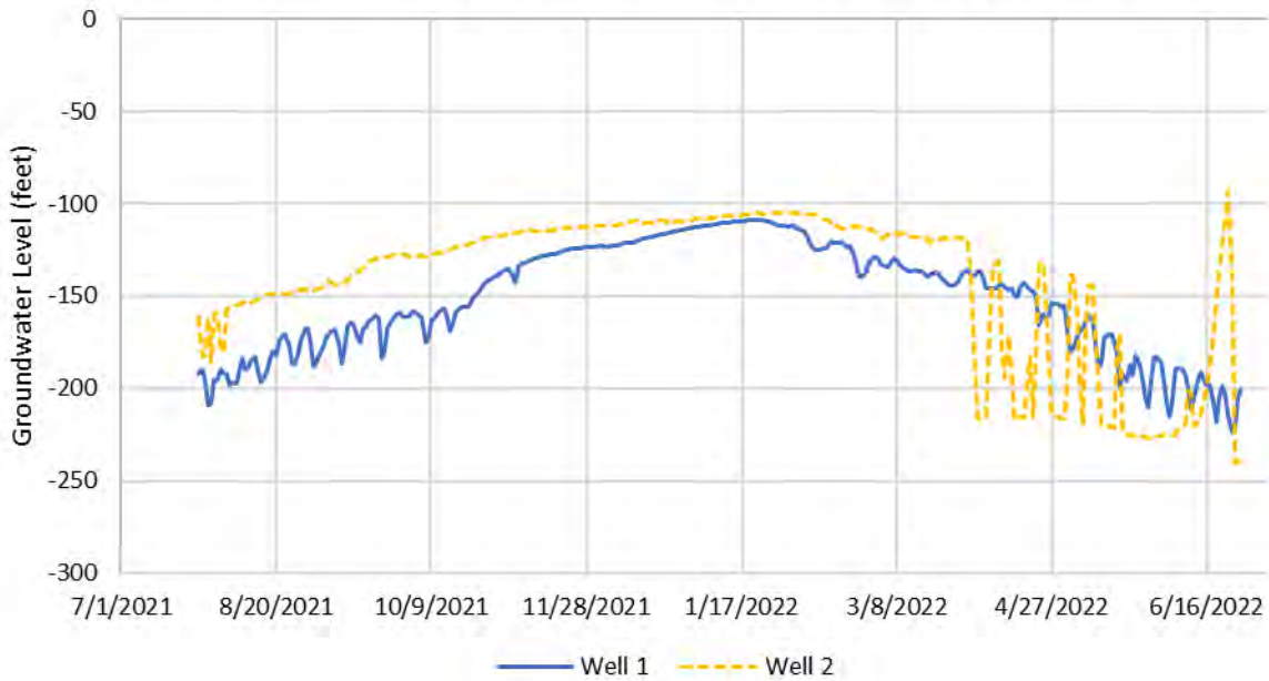
Figure 2. Groundwater levels at two sample wells from July 2021 through June 2022. The groundwater levels shown represent feet below the ground surface. The groundwater levels shown are both static (well off) and dynamic (well running), showing how the level draws down under operating conditions. Well 2 has a higher average water level, but more significant draw down than Well 1.
