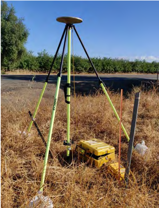
Static GPS receiver at H62U
